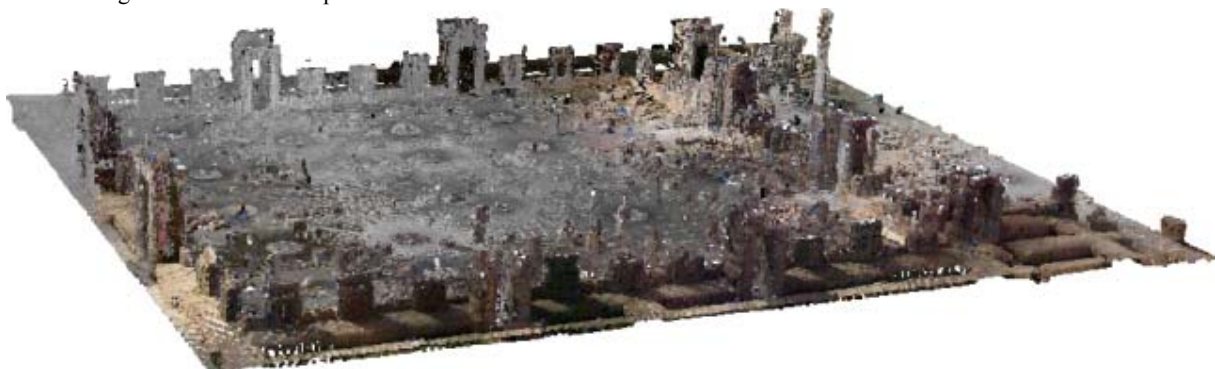
Hall of 100 Columns, 3D Point cloud of 57 merged true colour scans, re-sampled 0.3 m cube, created semi-automated while scanning, the grey areas were scanned during cloudy periods
